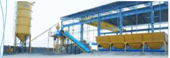
25 Cum to 120 Cumt. Batching Plant
