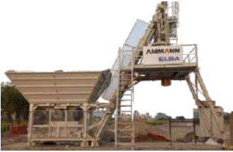
Concrete Batching Plant
